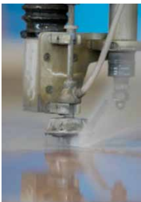
Figure 2. Photograph of AWJ (Courtesy of Stahl-Contor, Zürich, Switzerland).
